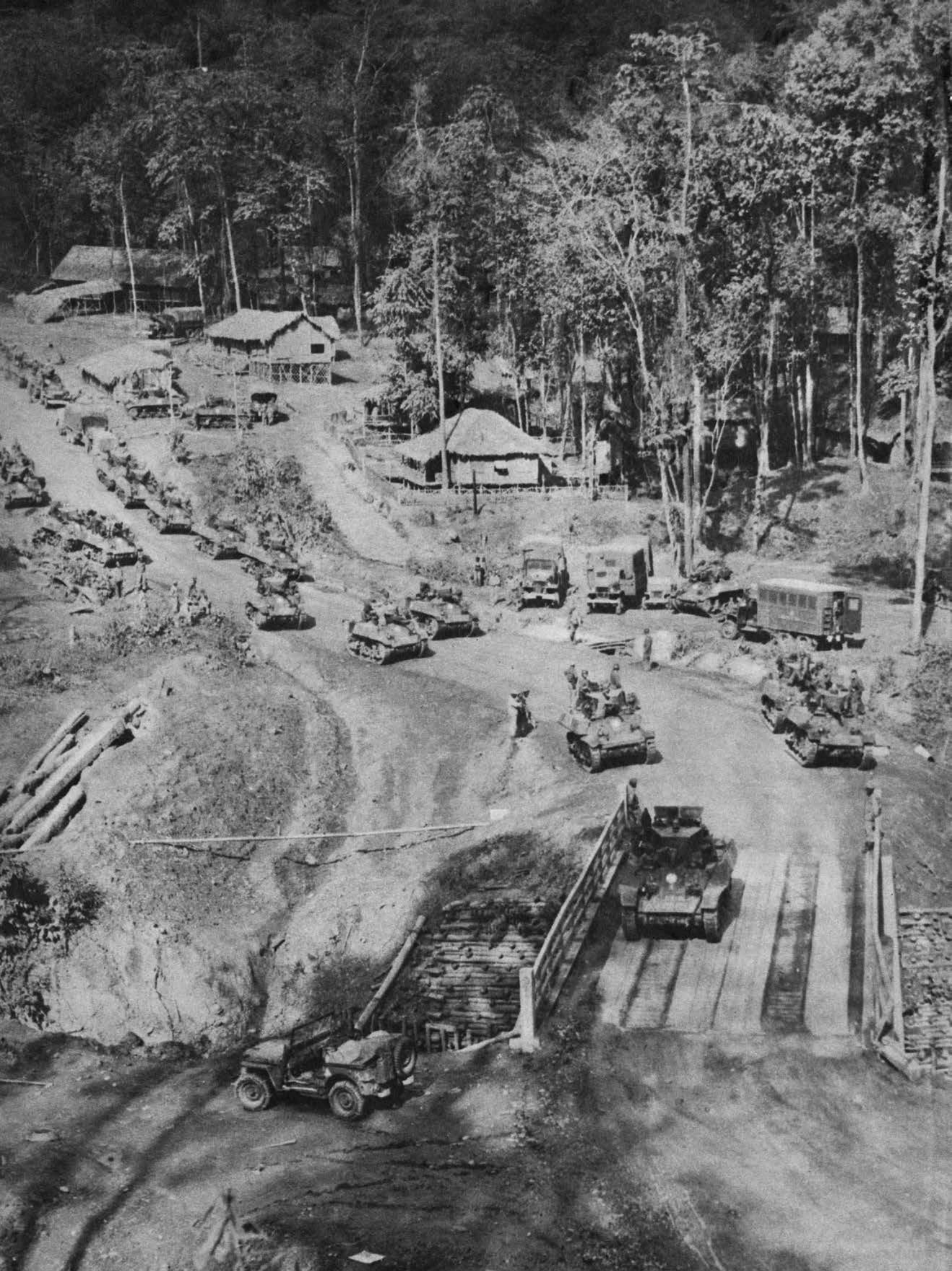
CHINESE-MANNED COLUMN OF M-5A1'S ROLLS DOWN LEDO ROAD. STANDARD U. S. LIGHT TANK, THE M-5A1 IS A TALL VEHICLE WITH A BOXY TURRET
